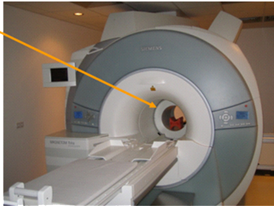
The MR/PET is comprised of a 3T Trio MRI into which a head-only PET insert is fitted. This unique arrangement allows the MRI and the PET to operate concurrently.
