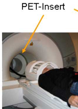
The MR/PET is comprised of a 3T Trio MRI into which a head-only PET insert is fitted. This unique arrangement allows the MRI and the PET to operate concurrently.
